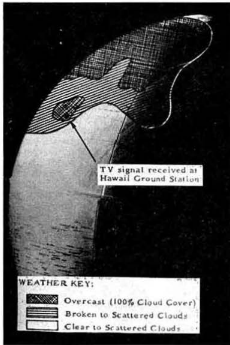
The lined areas at the left represent a cloud-cover map, prepared from meteorology charts which have been superimposed on a globe to show the lighted areas which the Explorer VI television scanner "saw" on August 14. As explained in the text, the scanning device resembles a television camera.
